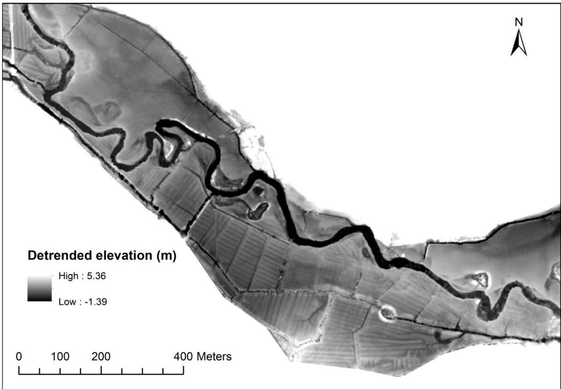
**Figure 6.3** A section of reach 17 where most of the floodplain surface has been subject to human modification
