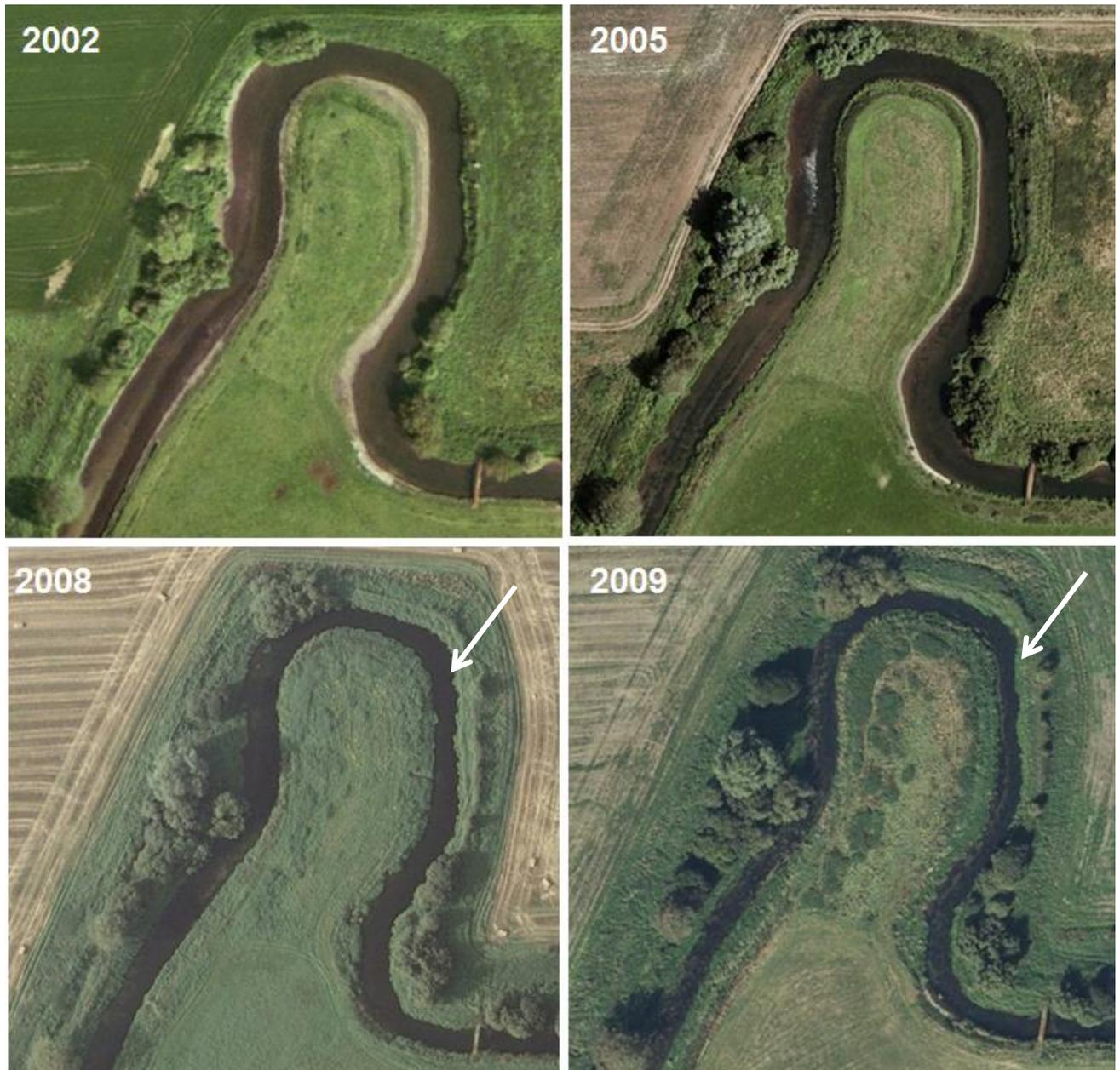
**Figure 4.40** Encroachment of the channel by marginal aquatic vegetation in Reach 12. (© Getmapping, Infoterra and Bluesky).
