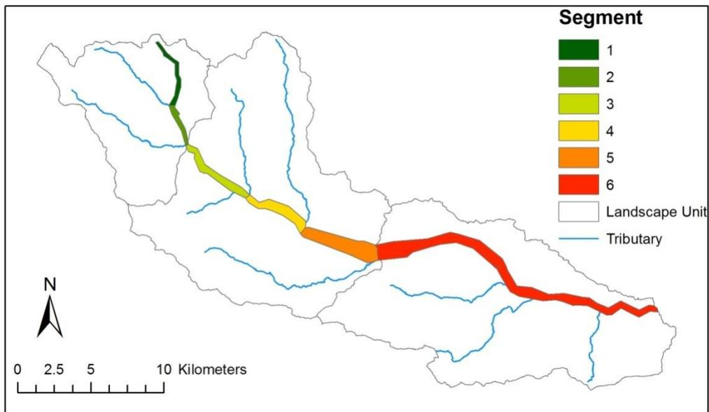
**Figure 3.8** The River Frome is delineated into 6 segments based on major changes in valley gradient, major confluences and valley confinement.
