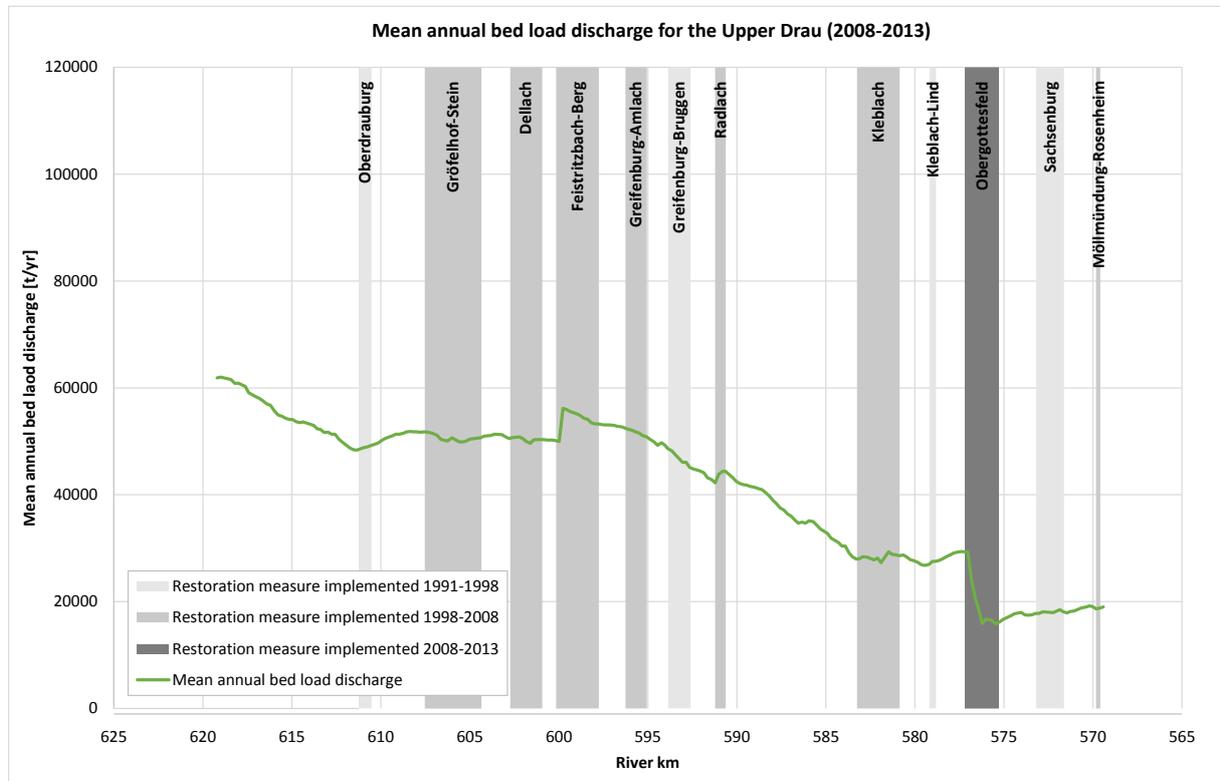
**Figure 7.5 Longitudinal variation of bedload transport at the Upper Drau River in the time period 2008-2013.**
