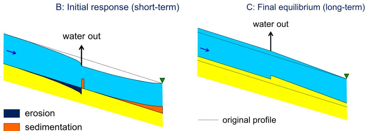
**Figure 2.3 Physics-based diagram of elementary short-term and long-term hydromorphological responses to water abstraction.**
