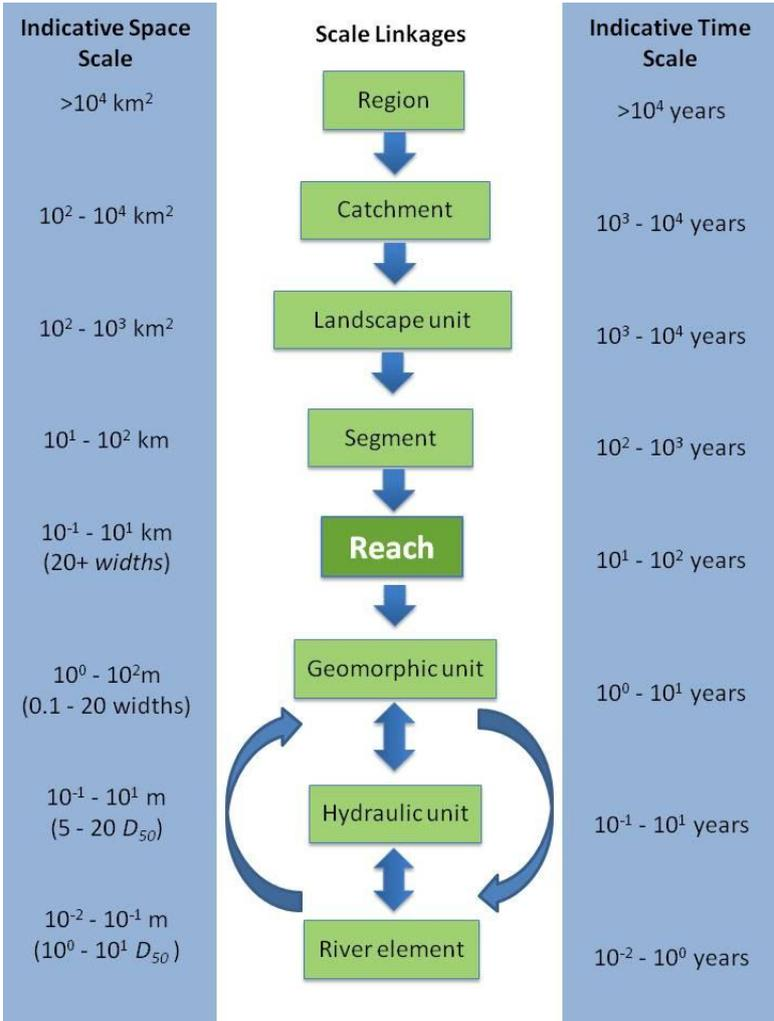
**Figure 2.5 Hierarchy of spatial scales for the European Framework, including indicative spatial dimensions and timescales over which these units are likely to persist.**
