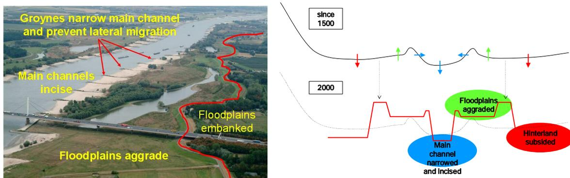
Figure 1.1 Aerial view of the Waal branch of the River Rhine (the Netherlands) showing several hydromorphological modifications and their impacts (left; photo: Bert Boekhoven) and a schematic presentation of the morphological changes (right; source: Van der Molen & Buijse 2005)
