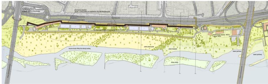
Figure 6.32. The Vistula River Park – conception of reconstruction of goyne’s system located on right bank of the river between two bridges: Lazienkowski and Poniatowski (Damiecki et al. 2008)
