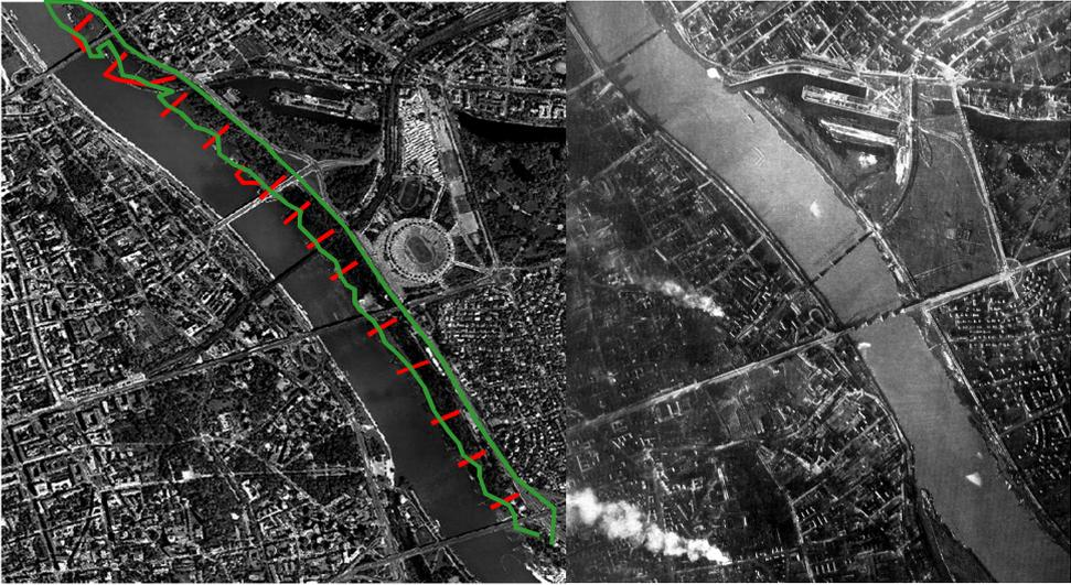
Figure 6.10. Aerial view of the Vistula riverbed in the city of Warsaw: left: in 1944 during the Warsaw Uprising in World War II, right: in 2006: red colour indicate location of goynes, green colour – area of sediment deposition and overgrow by high vegetation (Damiecki et al. 2008).
