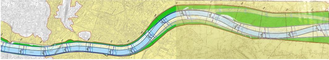
Figure 6.9. The Vistula River training works in project from 1960, executed in the 1970s of the XX century (Damiecki et al. 2008)
