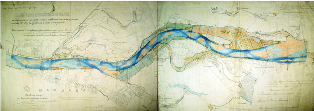
Figure 6.8. The project of the Vistula River training works made by Kostanecki in 1873, executed by Lindley in 1884 – 1889 as a part of the water supply infrastructure project in Warsaw (Damiecki i in. 2008).
