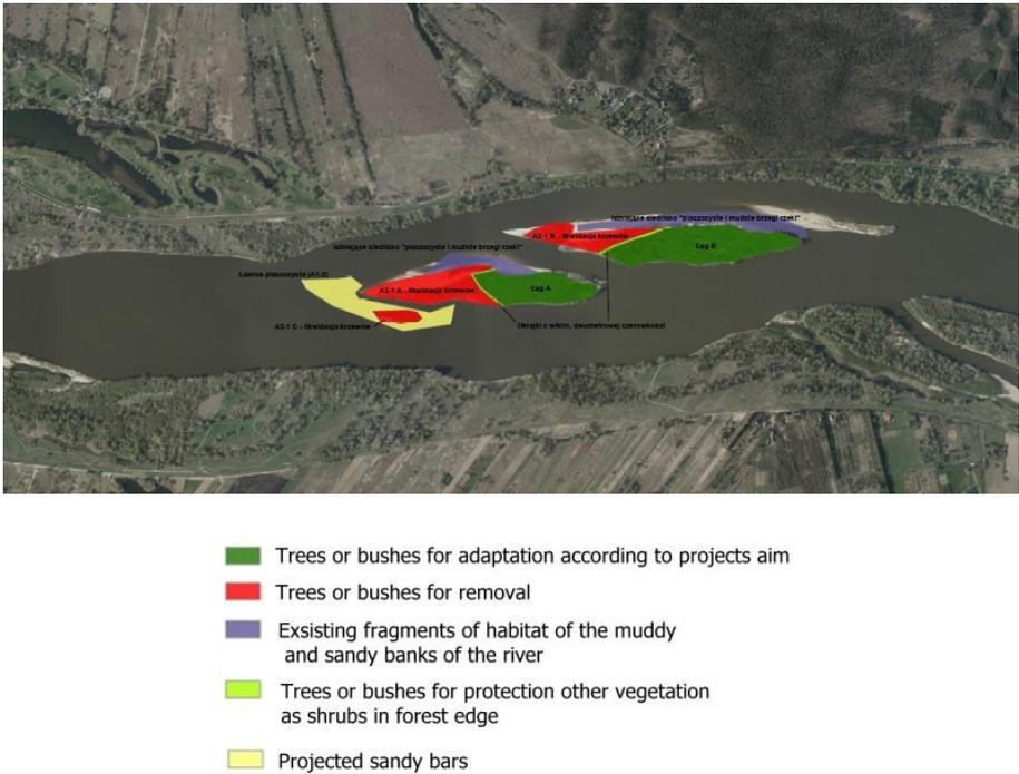
Figure 6.34. The scope of measures planned to use for restoration island on the „Lawice Kielpinskie” nature reserve area in km 527-538 (Halcrow 2013)
