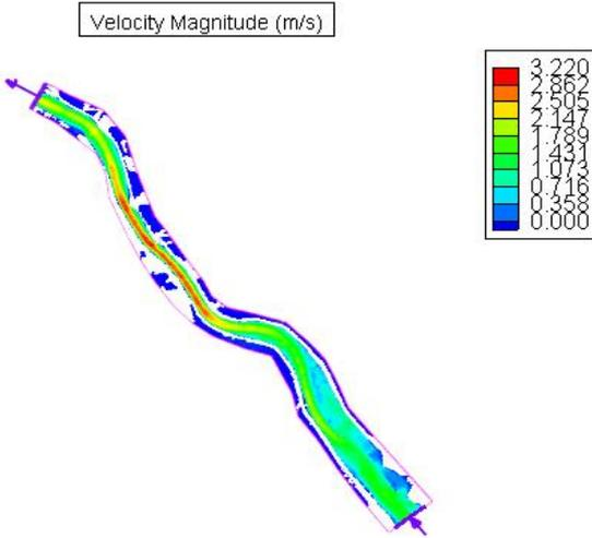
Figure 6.20. Variability of flow velocity during the 100-year flood flow on the Vistula River section in Warsaw – results of CCH2D hydrodynamic model calculation used for discharge  $Q_{p=1\%} = 7214 \text{ m}^3 \cdot \text{s}^{-1}$  (Magnuszewski et al. 2008)
