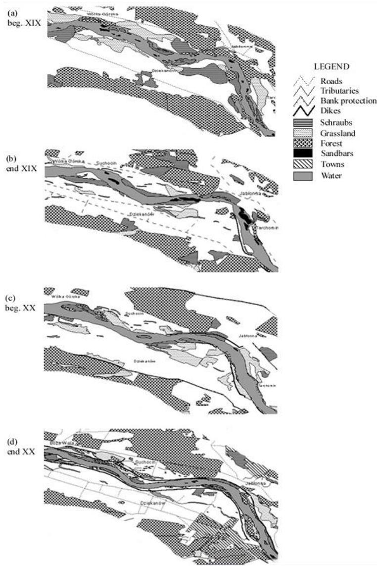
Figure 6.5. Changes in the Vistula riverbed on the reach Zeran – Boza Wola (km 525-545) in XIX (a,b) and XX (c,d) centuries (Zelazo et al. 2002).
