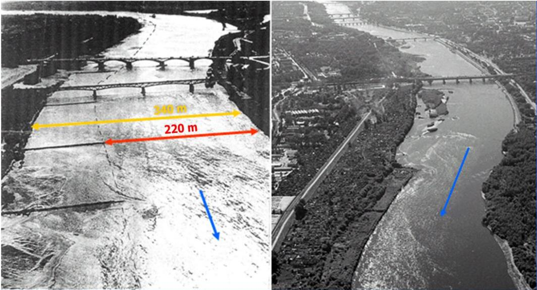
Figure 6.24. River training works in the Vistula riverbed in Warsaw. The left part: Aerial view of the groins system in 1964 - after completion of the project. The right part: Aerial view of the riverbed in 2006 – spaces between groins filled by sediments and covered by high vegetation.
