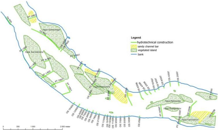
Figure 6.27. Planform of the Vistula riverbed and location of the hydrotechnical constructions in 1961 section of km 596-602: area of the nature reserves „Kępa Rakowska” i „Kępa Antoninowska” (Popek et al. 2009)
