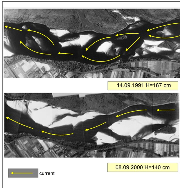
Figure 6.4. Changes of the riverbed sandy forms configuration upstream Warsaw on the Vistula River nature reserve “Wyspy Swiderskie” section in km 491-495, modified (Dobrowolski and Glowacka 2002).
