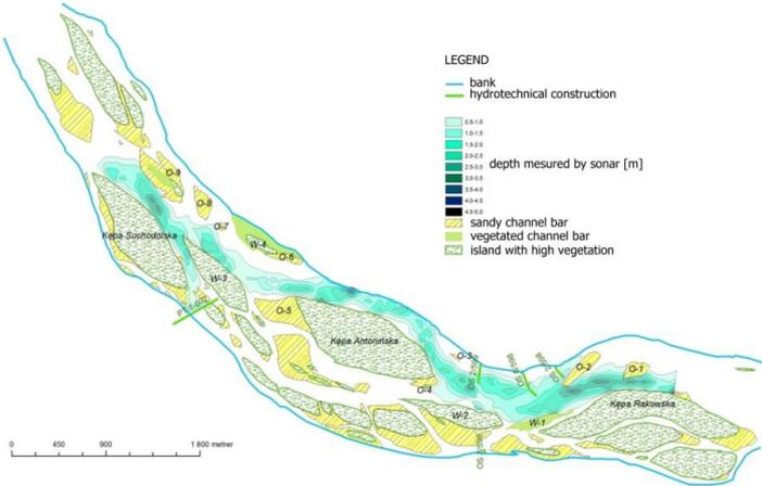
Figure 6.28. Planform of the Vistula riverbed and location of the hydrotechnical constructions in 2009, section of km 596-602: area of the nature reserves „Kępa Rakowska” i „Kępa Antoninowska” (Popek et al. 2009)
