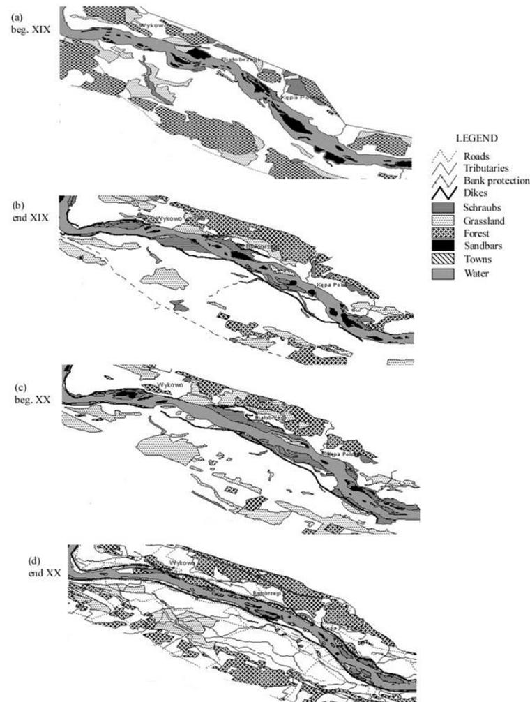
Figure 6.6. Changes in the Vistula riverbed on the reach Rakowo – Kepa Polska (km 598-622) in XIX (a,b) and XX (c,d) centuries (Zelazo et al. 2002)
