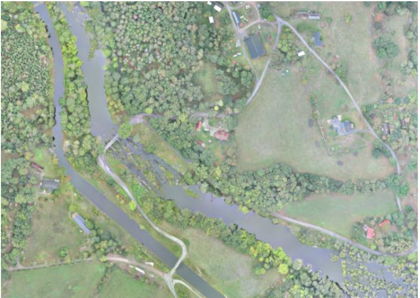
Figure 3 + Figure 4: Overview of parts of the restored stretch in River Mörrumsån (left), also visible is the man-made channel feeding the Hemsjö övre hydropower station. To the right a photo of a restored stretch during a flow episode when more than the dictated minimum flow of 1 m 3 /s has been directed through the natural channel. Salmonid spawning gravel was added here in 2010. Photos by Frauke Ecke, SLU.
