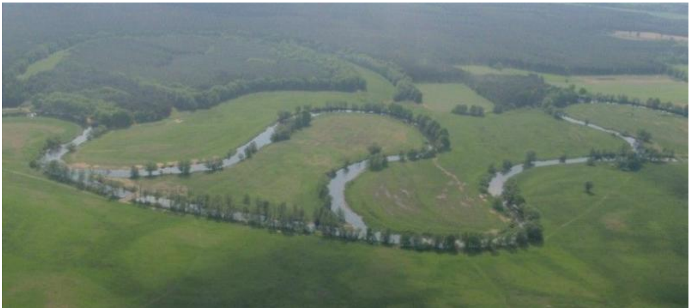
Figure 1: Re-meandering – the former backwater has been reconnected at both sides and the former main channel blocked by a dam (near the left, upstream opening) (photo: Isabell Hiekel).
