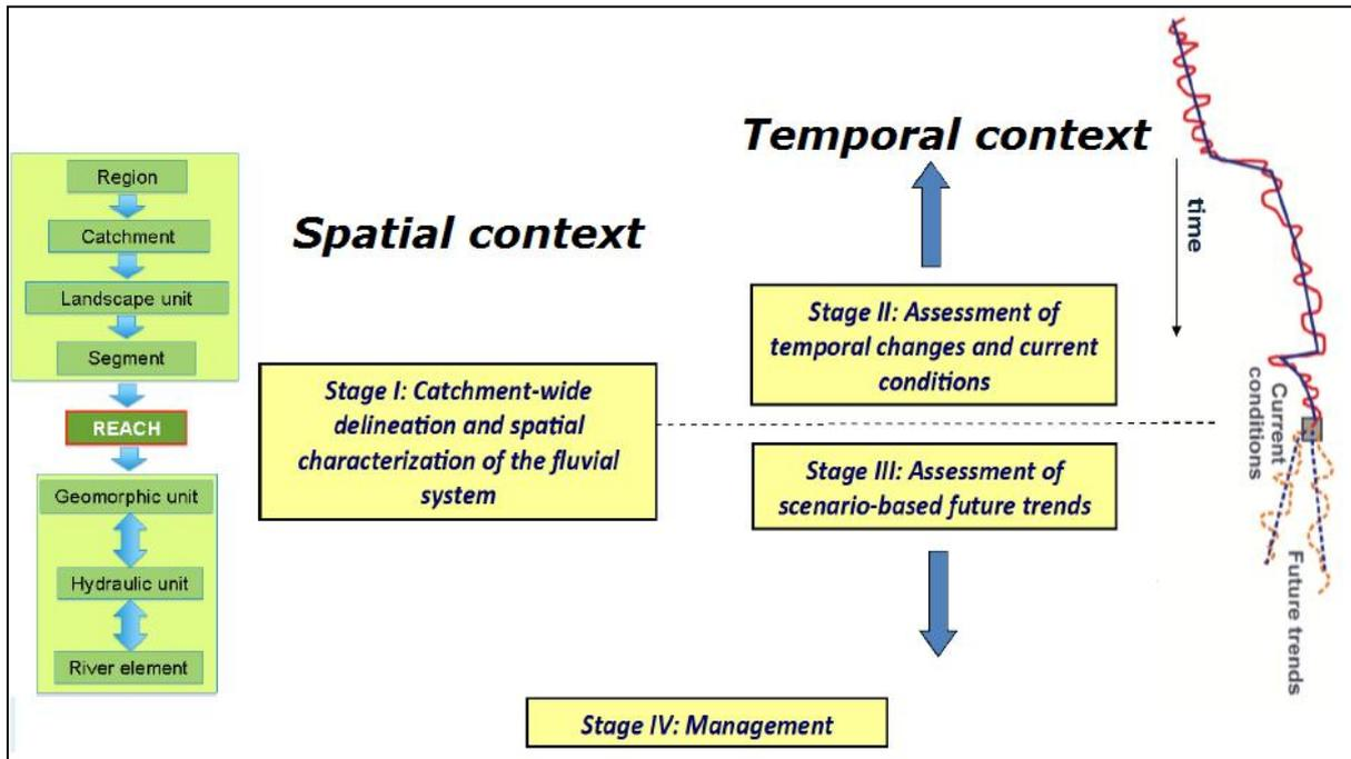
Figure 6 - Structure of the overall REFORM hydromorphological framework (Rinaldi et al. 2015). On the right side, the graph emphasises that the present state of the river system represents a spot within a long trajectory of evolution that needs to be known to understand current conditions and possible future trends. On the left side, the multi-scale hierarchical framework used for delineation and characterization of the fluvial system is presented (Gurnell et al. 2014).
