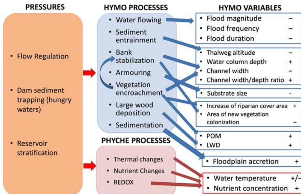
Figure 3.- Conceptual frame work of large dams and reservoirs effects on Hydromorphological (HYMO) and Physic-Chemical (PHYCHE) processes and variables (POM=Particulate Organic Matter; LWD=Large Woody Debris).
