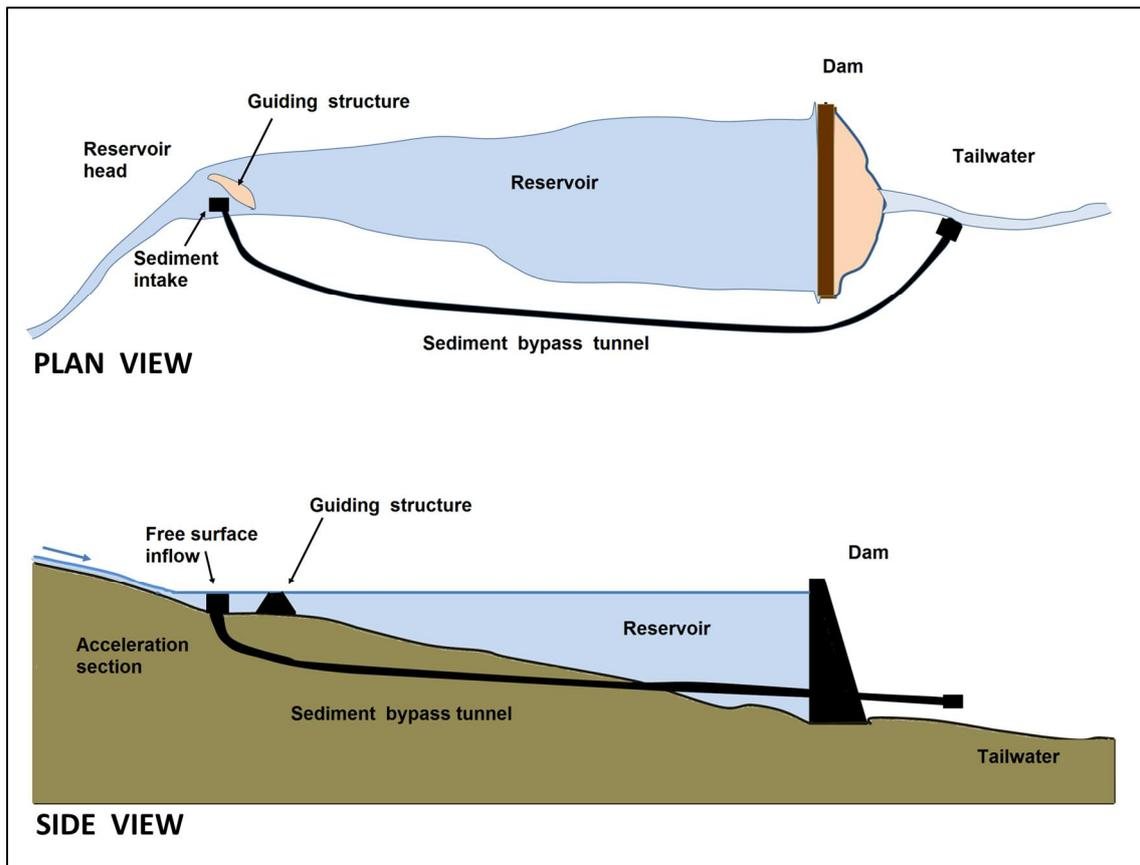
Figure 7.- Scheme of a sediment bypass tunnel system associated with a reservoir designed with the sediment intake located at the reservoir head under free surface conditions (based on Auel & Boess, 2012).
