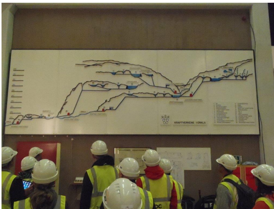
Figure 2.4. The by-pass scheme of a hydropower plant in Norway. The by-pass runs through the mountains (Photo: Tom Buijse).
